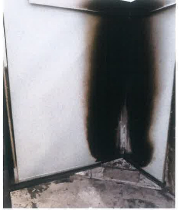
Photograhp 8. Corner detail of Sample 1 (After test)
